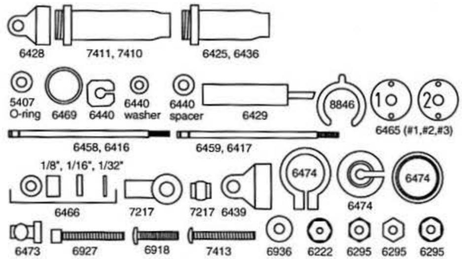
**GOLD. ASSOCIATED'S STANDARD SHOCKS (#6420-#6429) ARE PRECISION MACHINED TO VERY CLOSE TOLERANCES.**
